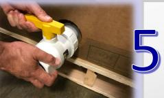
The valve is ready to connect to the outbound couplings to drain the liquid contents. **Note: Support the valve assembly at all times and keep protected from trauma and or abuse.**
