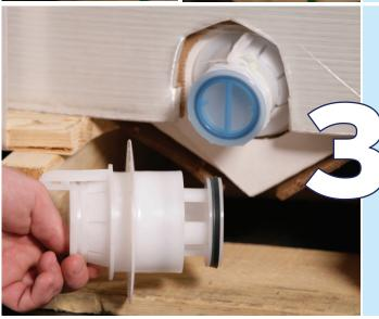
Remove safety tie strap. When ready to drain, lift locking finger and push "EZ-VALVE" body in to initiate flow. Side profile of valve assembly shown here for reference. Then use locking finger to secure "EZ-VALVE" in the open position for continuous evacuation. To stop flow, pull EZ-VALVE out and return the valve to the closed position. Note: Make sure to support or brace "EZ-VALVE" at all times and keep protected from trauma and or abuse.
