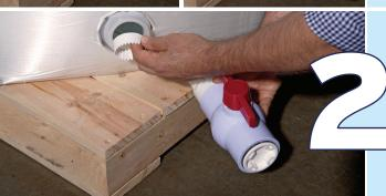
Remove the 2" disposable ring cutter from the evacuation fitment. Turn the ball valve handle to the open position so the valve handle is in alignment with the valve body. The valve must be in this (OPEN) position in order to clear the corner of the pallet during installation.
