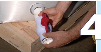
Thread the ball valve assembly into the bottom 2" evacuation fitment. As the valve assembly is threaded into place, the increased thread engagement will cause the disposable cutter to pierce the membrane. NOTE: It is very important to thread in the valve assembly all the way to make sure the o-ring is seated and sealed against the evacuation fitment.
