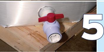
Ball valve handle is returned to the closed position and ready to connect to outbound couplings to drain the liquid contents. Note: Support valve assembly at all times and keep protected from trauma and or abuse.
