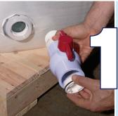
Remove the 2" screw cap from the bottom 2" flange of the bag liner. Screw this same 2" cap into the outbound side of the ball valve.
